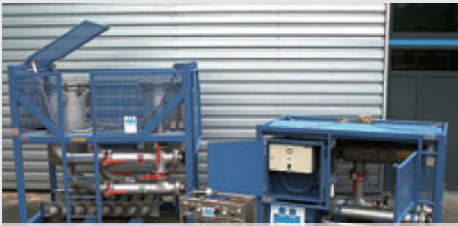
Temporary Water Injection, Offshore Qatar, 120m 3 /hr, 50 micron, polish filtration 2 micron
